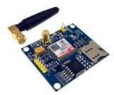
• Input voltage range 5V-20V DC, power supply range for a variety of power supply applications.
