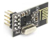
• Maximum operating speeds up to 2Mbps, GFSK modulation efficiency, Anti-interference ability,
