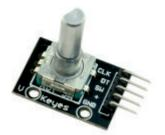
• A 360 Degree Rotary Encoder is a Bread Board Friendly extremely precise module that provides an indication of how much the knob has been rotated AND what direction it is rotating in.
