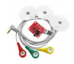
• AD8232 adopts double poles high-pass filter to eliminate the motion artifacts and electrode half-cell potential
